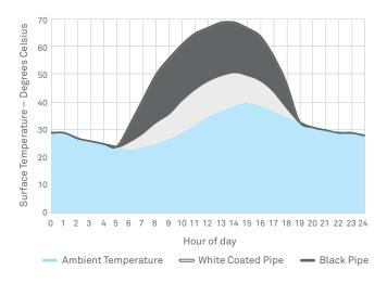
Figure 2. Typical thermal effects of solar radiation on white coated pipe and black pipe over 24 hours
